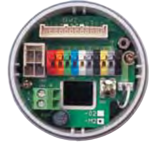
Color Coded Wiring Terminals
